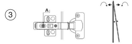
Adjusting the angle of the door.Loosen screw'A' and slide the hinge arm either forwards or backwards until the door is vertical then tighten screw'A'.
