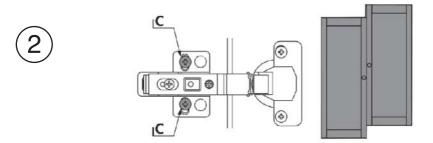
Adjusting the height of the doors. Loosen screws 'C' then slide the hingeplates up or down until the doors are even then tighten the screws.
