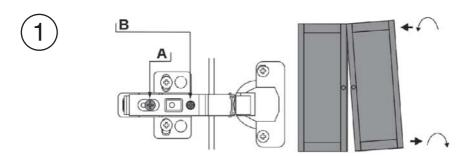
Adjusting the gap between the doors. Loosen screw 'A' slightly. Turn Screw 'B' clockwise to move the door away from the side, turn anti-clockwise to move the door towards the side. When gap is equal tighten screw 'A'.
