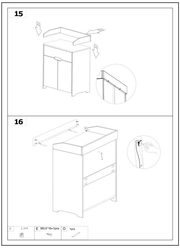
There is an anti-topple strap fixed to the back of the chest. Choose a suitable wall fixing and then fasten the strap to the wall as shown using the appropriate fixings.
