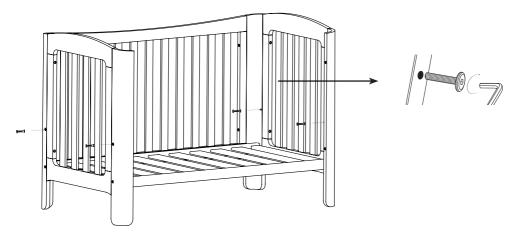
STEP 5 Assemble remaining fixed side using 4 x 60mm bolts
